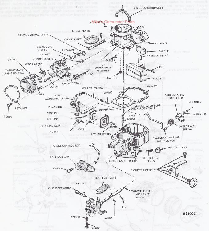
FORD SINGLE BARREL CARBURETOR ASSEMBLY (PISTON TYPE AUTOMATIC CHOKE)
