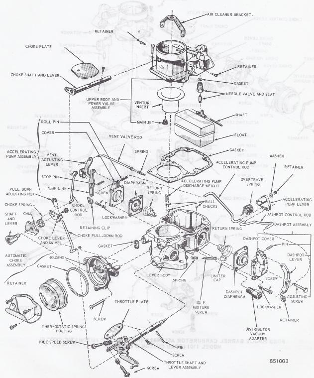
FORD SINGLE BARREL CARBURETOR ASSEMBLY (SPRING TYPE AUTOMATIC CHOKE)
